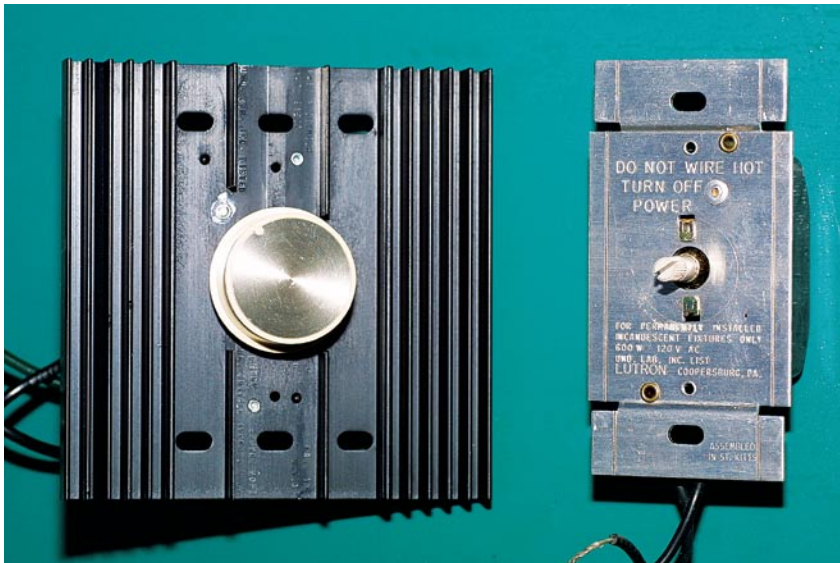
Although more expensive, the larger 1,500-watt dimmer (left) has a large heat sink, enabling it to handle more lights and last longer than the standard 600-watt dimmer (right).
